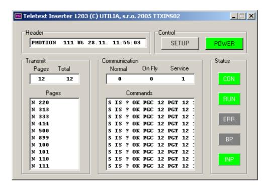
Status area indicates incidental troubles of inserter card by red color. **CON**=no connection to card, **RUN**=not active, **ERR**=internal error, **BP**=bypass, **INP**=no video in. *Do not click POWER button, it will close TTXIns and stop all teletext transmission!*
