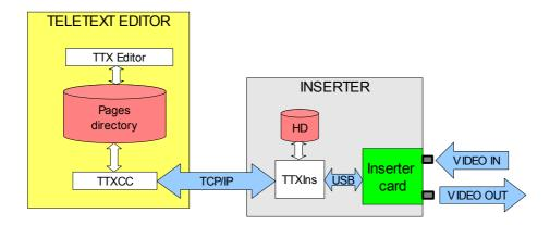
Inserter card is controlled by **TTXIns**. This program also generates **Page Header**, provides diagnostic and Inserter setup. Inserter system clock is used for page header time and date.
