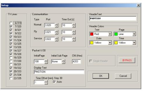
Checkboxes at **TV Lines** numbers signs real TV line numbers in which you want to transmit teletext data. It is good idea to consult this setting with responsible personal to prevent conflict of some other VBI signals. Typical TV Lines settings is on this image. You should also set up properties of the header in upper right corner of the SETUP window Important is a **Header Text**, usually the name of TV station or teletext entrepreneur.
